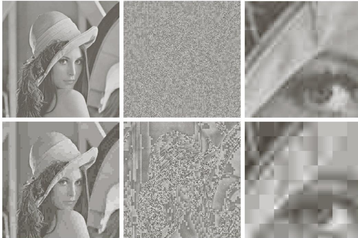
FIGURE 8.32 Two JPEG approximations of Fig. 8.9(a). Each row contains a result after compression and reconstruction, the scaled difference between the result and the original image, and a zoomed portion of the reconstructed image.
